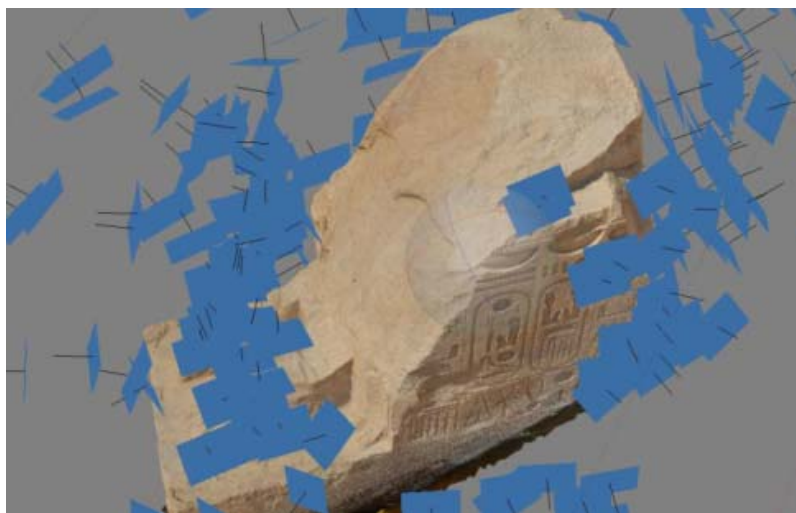
Photo 14 Series of photos taken by the camera (blue squares) to generate the 3D model of the Colossus found in the Temple of Heryshef
