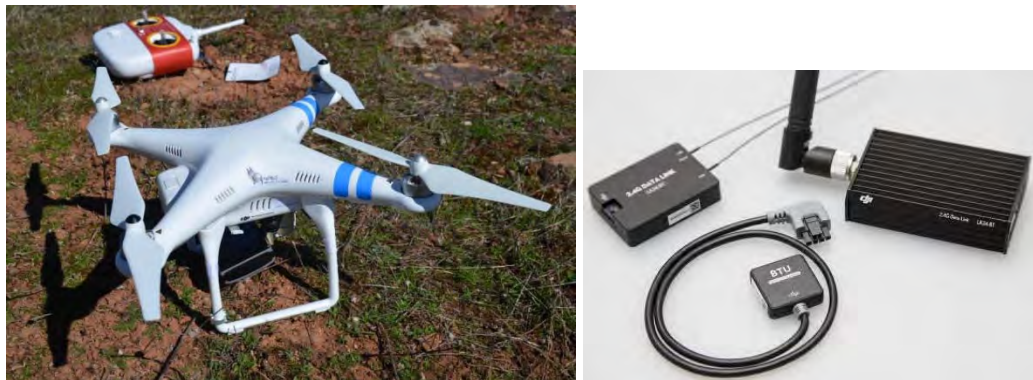
Photo 13 a and b. Drone cuadricóptero DJI PHANTOM2 with gimbal zenmuse H3-2D for cameras gopro hero3. And Inhalambric conexions for the control of the Drone.
